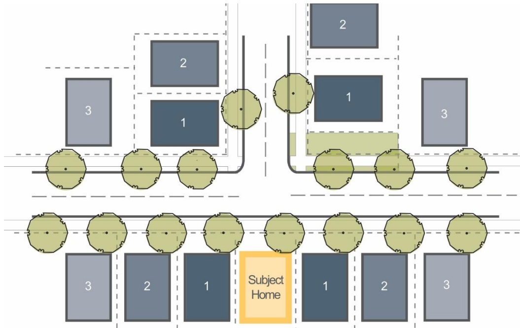
Chapter 6 Image 2 This example shows how the anti-monotony standards are applied at an intersection with common area shown in green between the subject lot and another.
