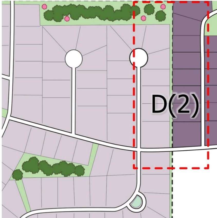
Chapter 2 Image 5. Perimeter lots must meet the width and/or size of adjacent neighborhood lots, depending on the amount of common area separating the neighborhoods. Other buffering may also apply in the landscape section.
